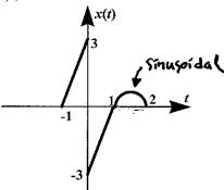
Problem 2: (*Laplace transform*) Determine the Laplace transform of the following signal, x(t), with only *ten* periods (cycles). (Note that the maximum amplitude is V with period T)
